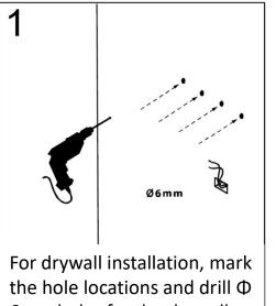
the hole locations and drill  $\Phi$ 6mm holes for the drywall anchors. Install a junction box behind the mirror for power connections.
