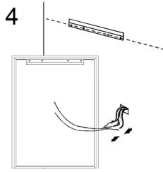
Connect the load (black) wire of the Dimming driver cable (white) to wall switch if used, otherwise to a common hot wire. Connect the load (black) wire of the Touch Switch cable (black) to hot wire.
